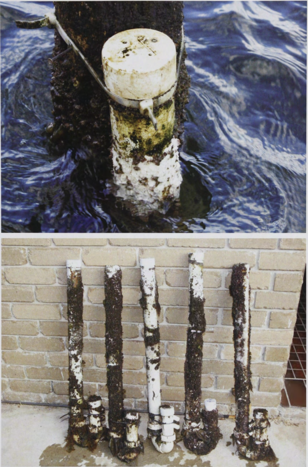
Figure 5.5: PVC pipe clay experiments in the estuary (above), and retrieved (below).
