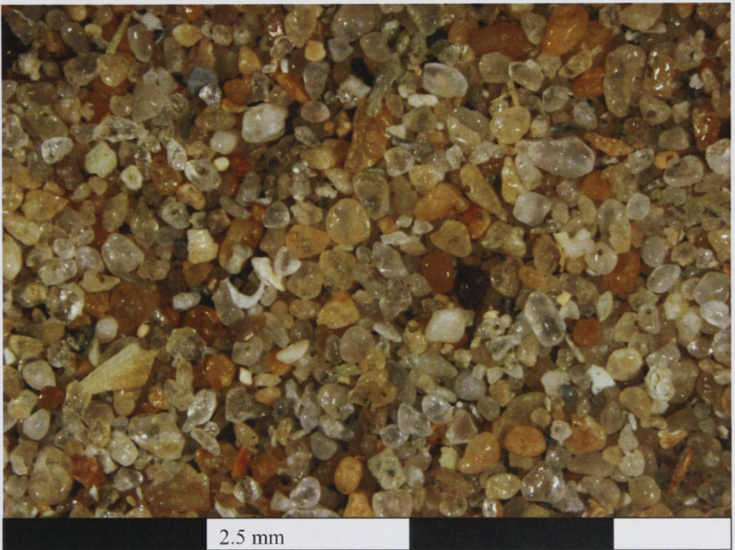
Figure 4.2: Well rounded quartz sand from Merimbula Beach. Minor fragments of carbonate are seen amongst the variably coloured and iron stained quartz grains.
