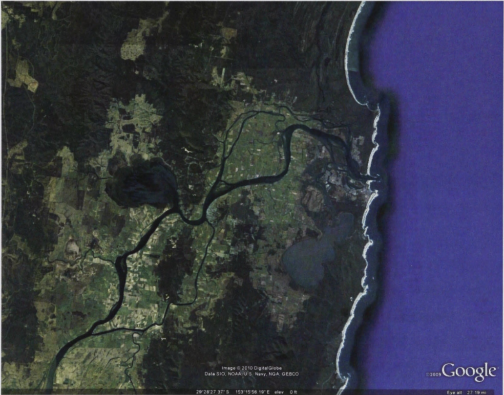
Figure 2.15: Clarence River, NSW – an example of a wave-dominated estuary where there is a small tidal influence
