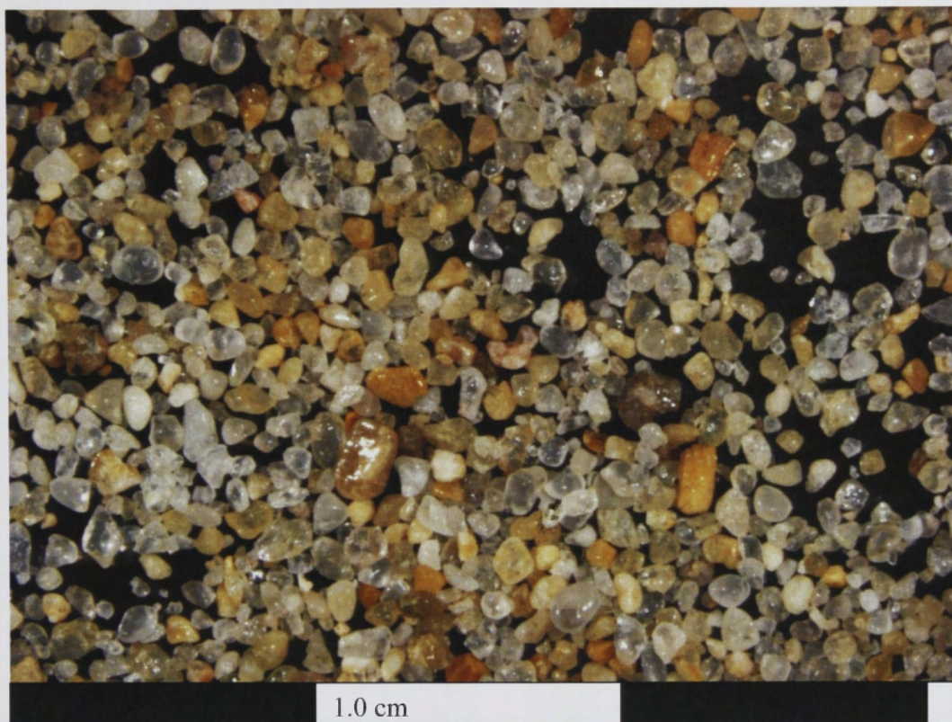
Figure 4.9: Grey sand that was treated with weak nitric acid and reverted to yellow sand, preserving the variable intensities of the surface sand yellow iron coatings.
