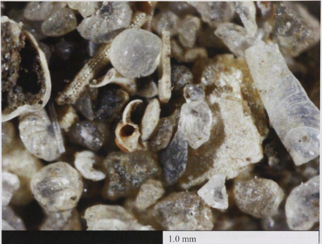
Figure 4.5: Merimbula Top Lake bottom sediment revealing broken echinoid pieces as well as foraminifera shells and some angular quartz grains.
