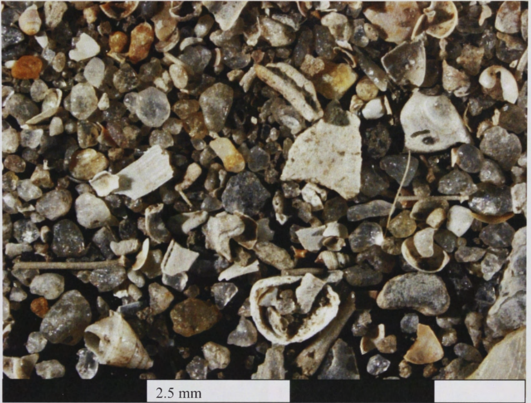
Figure 4.4: Sediment from Merimbula Top Lake (sampled from deeper water below tidal range). Note the well rounded quartz grains of variable colour, together with fragments of various bivalves and gastropod shells.
