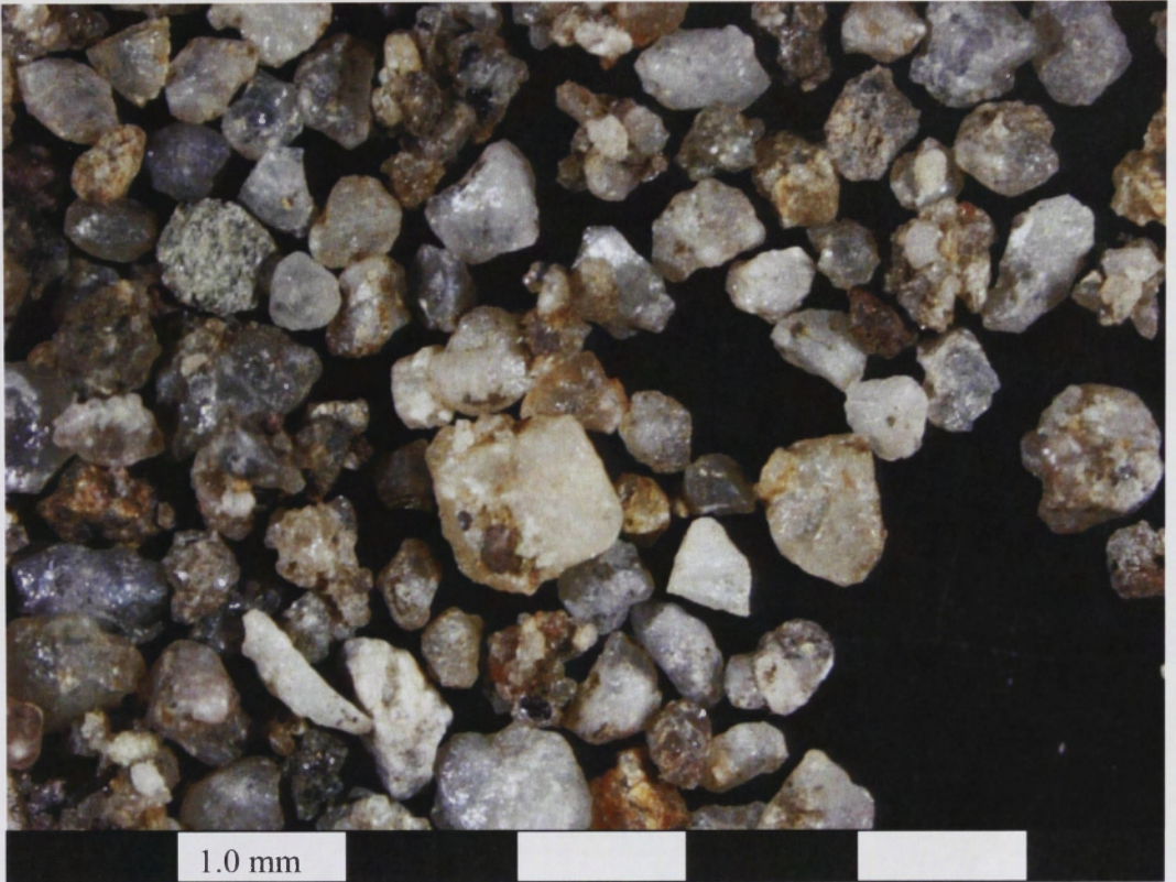
Figure 4.3: Poorly sorted angular to subrounded quartz and pink feldspar grains deposited from Millingandi Creek where it flows into Merimbula Lake.
